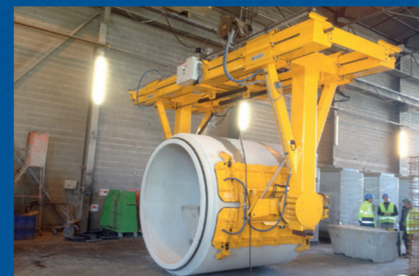
Demoulding turning beam
