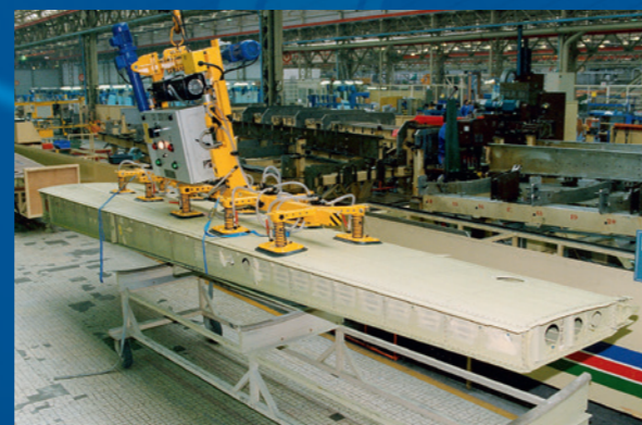
Vacuum beam for aluminium plate application
